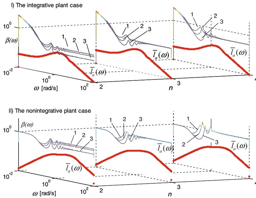
Fig. 2 Influence of disturbance observer parameters on the robust stability – 1  $T_o = 9$ , 2  $T_o = 6$ , 3  $T_o = 3$
