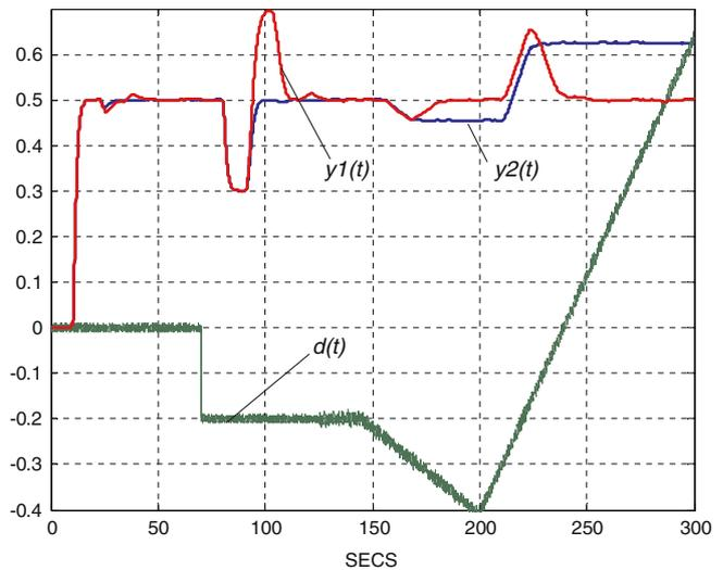
Fig. 4 The response of the structure with non-integrative plant and PI main controller (10) with ( $y_1$ ) and without ( $y_2$ ) local minor loop
